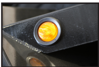
Sealed beam lighting
